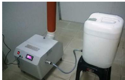
Gambar 1: Pelembapan jenis ultrasonic ( ultrasonic humidifier )
