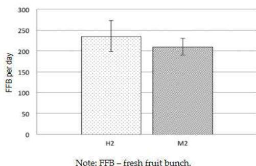
Figure 4. Average productivity per day for the cutting only harvesting machine without a bucket (H2) and manual harvesting without transportation (M2).
