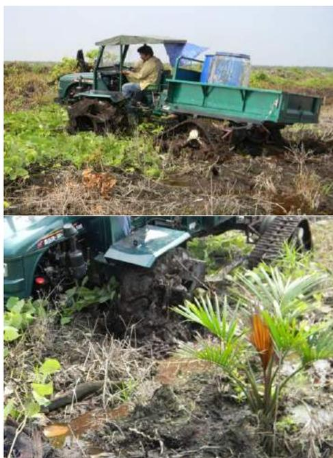
*Figure 5: Field test conducted at peat area with load*
