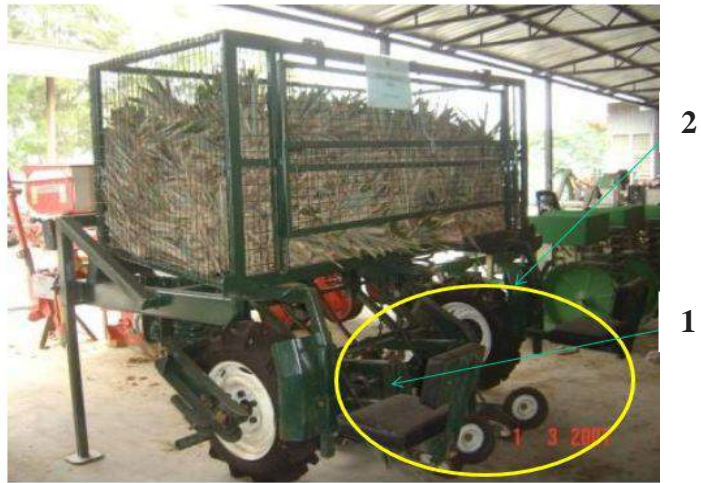
Figure 4: The manual/semi-auto pineapple transplanter (1) operator seat at the lower back of the machine- safety Issue (2) Speed of the feeding mechanism missing point
