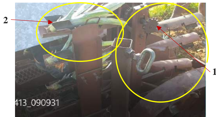
Figure 6: Show (1) the gripper mechanism was too fast because it depended on the wheels from the tractor's travel speed. (2) show that the pineapple sucker is a bit bigger than the gripper
