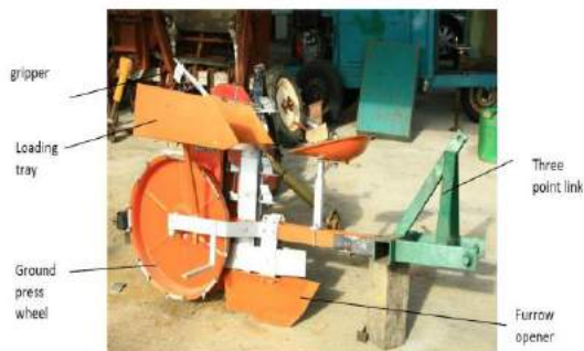
Figure 2 gripper type mechanical transplanter
