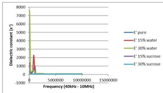
Figure 5: The dielectric properties of pure honey, honey adulterated with sucrose and water at frequency range from 40kHz to 10MHz
