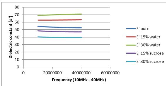
Figure 6: The dielectric properties of pure honey, honey adulterated with sucrose and water at frequency range from 10MHz to 40 MHz
