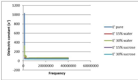
Figure 4: The dielectric properties of pure honey, honey adulterated with sucrose and water at frequency range from 40kHz to 40 MHz
