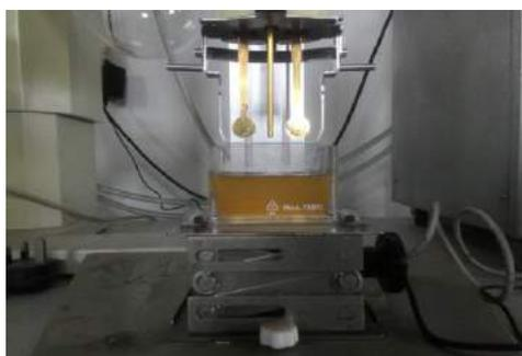
Figure 3: The honey sample inside viscometer cup
