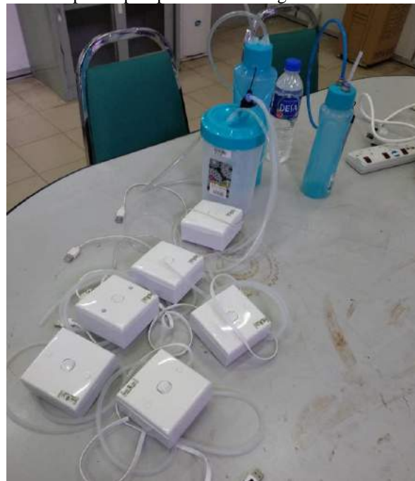
Figure I. The completed homemade stingless bee pumps showing six pump boxes and three storage bottles.
