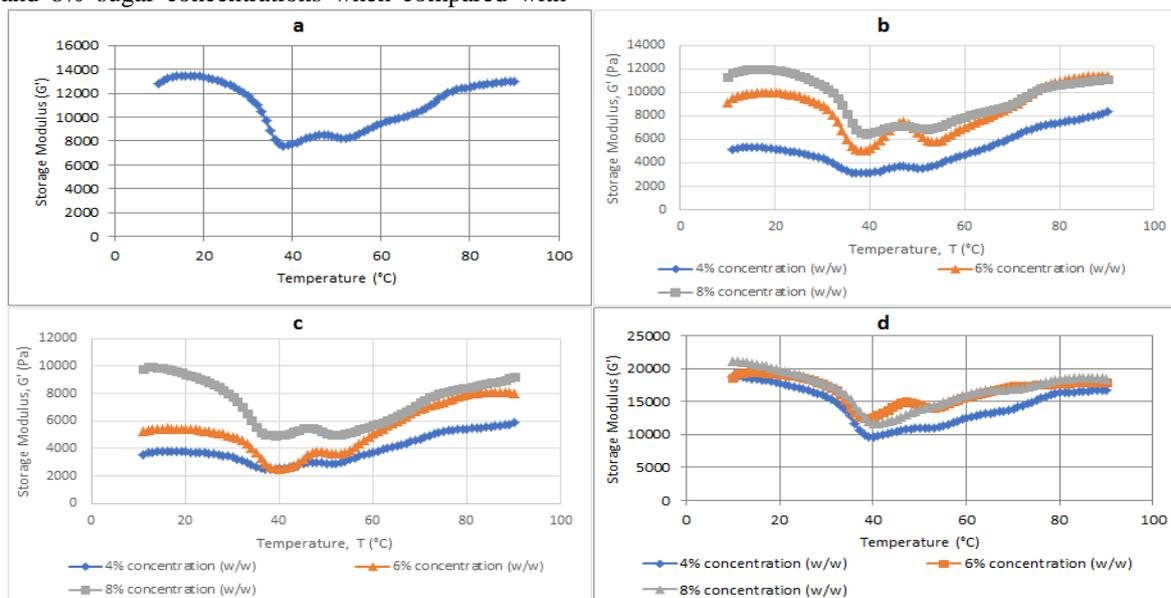
**Figure 2: The storage modulus ( $G'$ ) for (a) control fish mince and fish mince added with (b) sucrose, (c) sorbitol, (d) mannitol at 4%, 6% and 8% (w/w) concentration subjected to temperature sweep**
