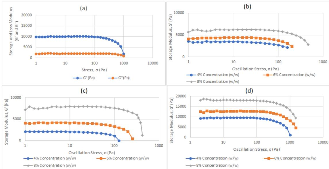
**Figure 1: The storage modulus ( $G'$ ) for fish mince added with (a) control, (b) sucrose, (c) sorbitol, (d) mannitol at 4%, 6% and 8% (w/w) concentration subjected to stress sweep**
