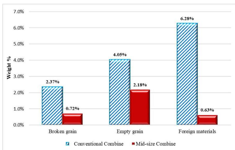
Figure 3. Quality of output grain for conventional and mid-size combine harvesters
