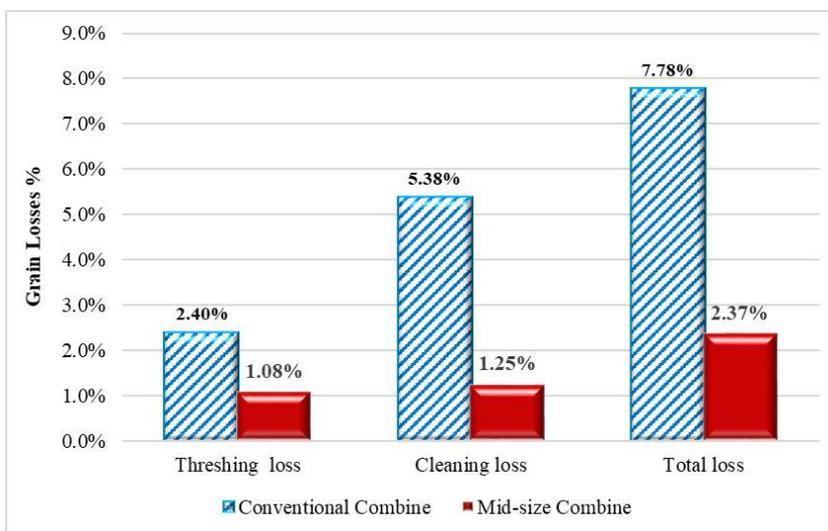
Figure 5. Total, threshing and cleaning losses of the conventional and mid-size combine harvesters
