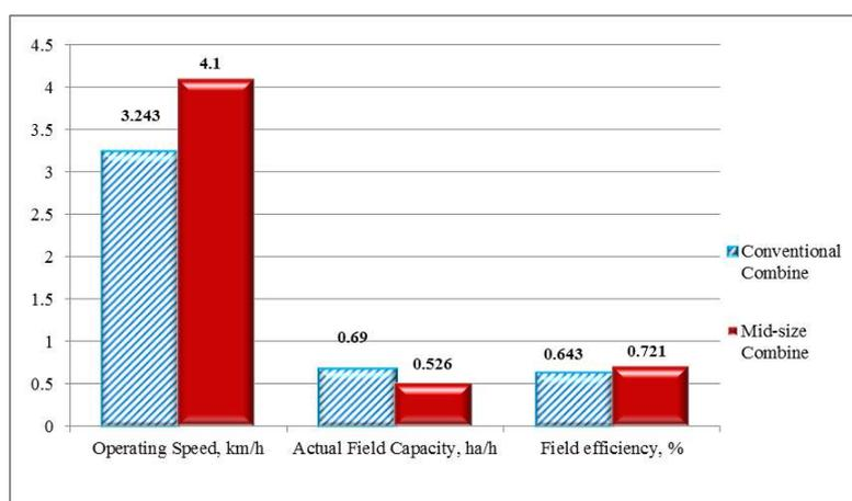
Figure 2: Comparison of field performances between Conventional and mid-size combines
