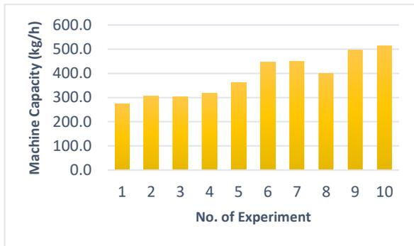
Figure 3: Results of Machine Capacity for Young Coconut Husk Processing Machine
