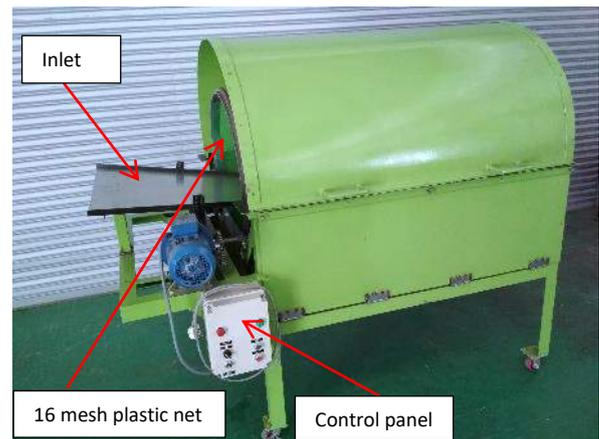
Figure 2: Rotary Screener for Filtering Process of Cocopeat
