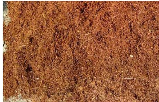
Figure 4: Extracted cocopeat before screening process
