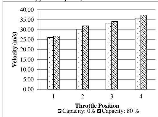
Figure 4: Air velocity at nozzle for different fruit capacities
