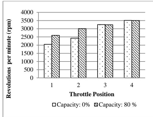
Figure 3: Comparison of blower fan speed at 0% and 80% of fruits capacity.
