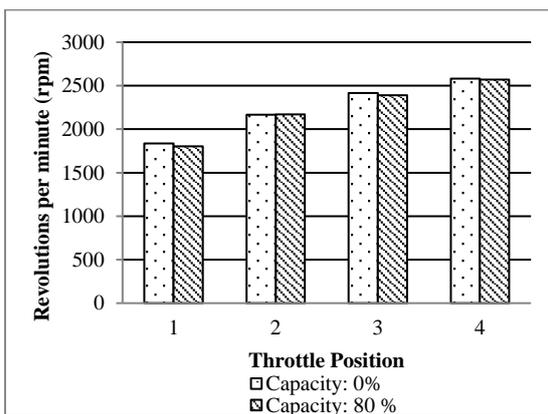
Figure 2: Comparison of engine speed at 0% and 80% fruits capacity.
