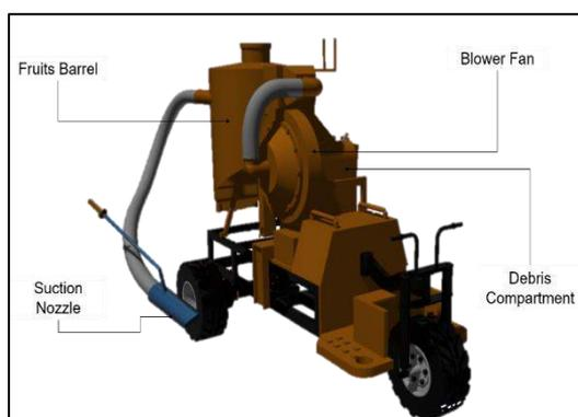
Figure 1: The isometric view of the machine.
