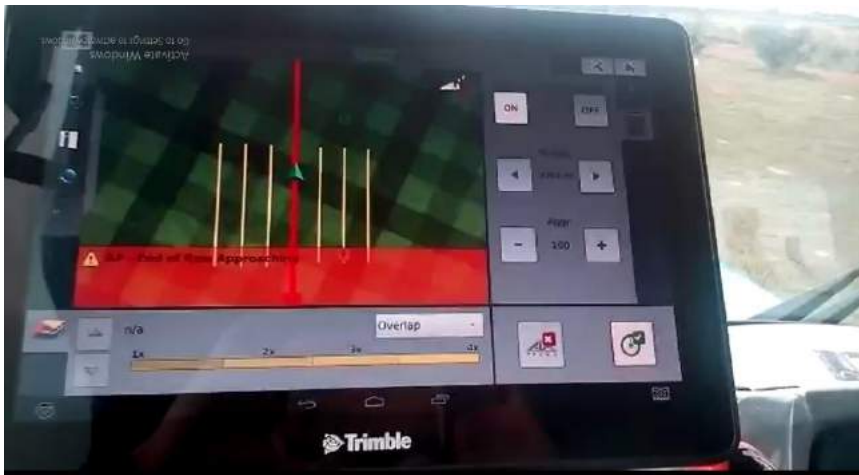
Figure 1. The GPS system of autopilot mode has been setup for tracking the straight-lines routes in the field
