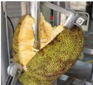
Figure 2: Cutting and splitting process by Vertijack
