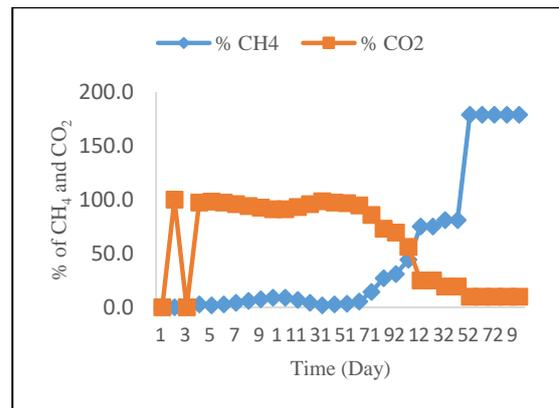
Figure 7(c): Methane and CO<sub>2</sub> at ratio 1:1
