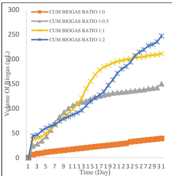
Figure 2: Cumulative biogas production for 30 days
