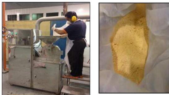
Figure 8: Grinding dried cut-strip Vitato into powder using Hammermill machine
