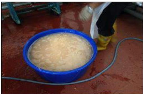
Figure 6: Soaking and tossing process of cut-strip Vitato using sodium metabisulphate
