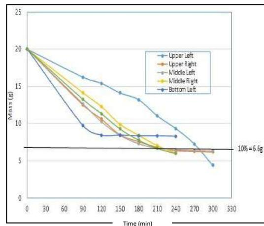
Figure 9: Mass reduction during drying of Vitato cut-strip
