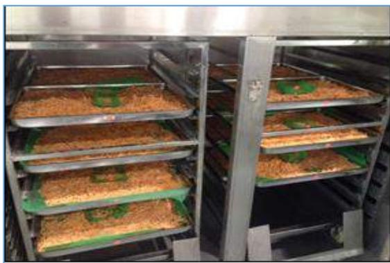
Figure 7: Drying process of cut-strip Vitato using cabinet dryer
