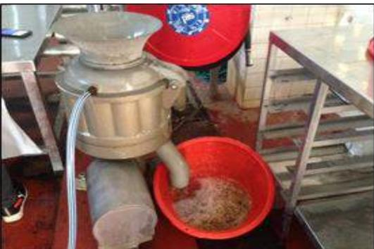
Figure 3: Deskinning and peeling process of Vitato using stone grinder machine
