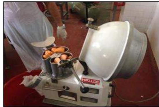
Figure 5: Slicing Vitato into cut-strip form using slicer machine
