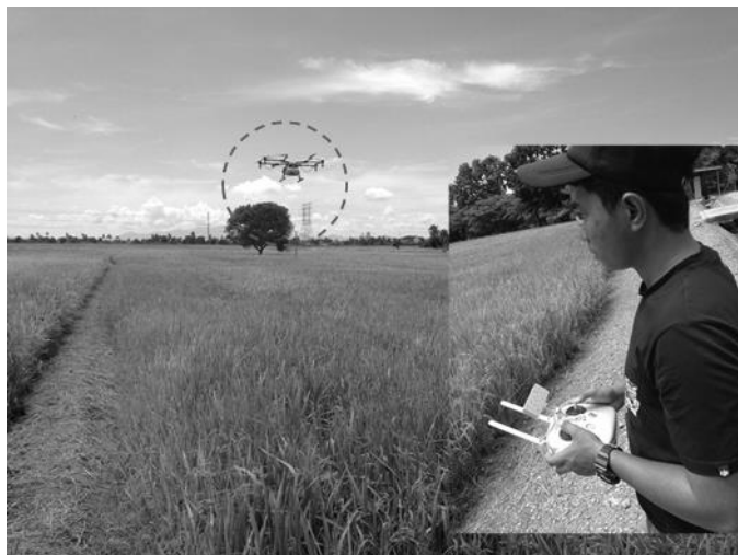
Figure 1: The pilot operates the DJI Agras-1 with semi-automatic control mode at the required flying height, deployed to perform the spraying test
