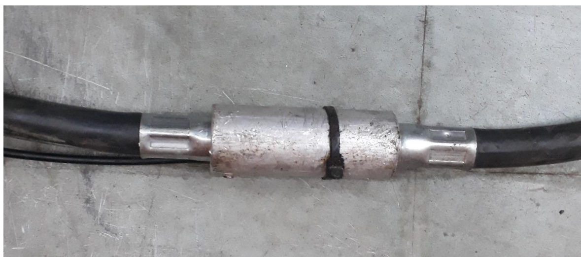
Figure 2: The connecting bush between the flexible shaft drive
