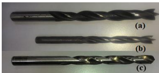
Figure 4: Drill bit used in the test; (a) 11 mm drill bit for wood purpose, (b) 8 mm drill bit for wood purpose and (c) 8 mm drill bit for general purpose
